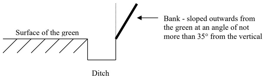
All new banks that are constructed, and all existing banks that are replaced, must meet the standard described in either diagram B.1.1 or diagram B.1.2 above, which was adopted with the introduction of the first Crystal Mark Edition of the Laws of the Sport of Bowls. The standard described in diagram B.1.3 above applies only to existing banks constructed before 2007.
